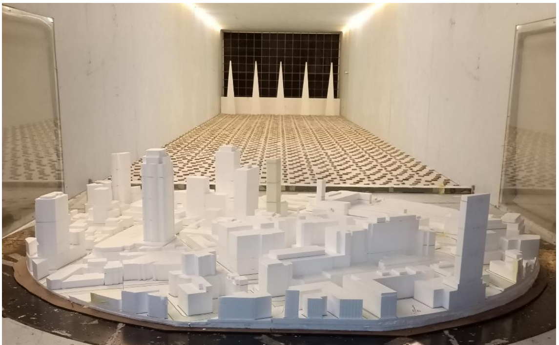
Figure 1d: Close up photograph of the Wind Tunnel Model (Proposed DCP Envelope, view from the west)
