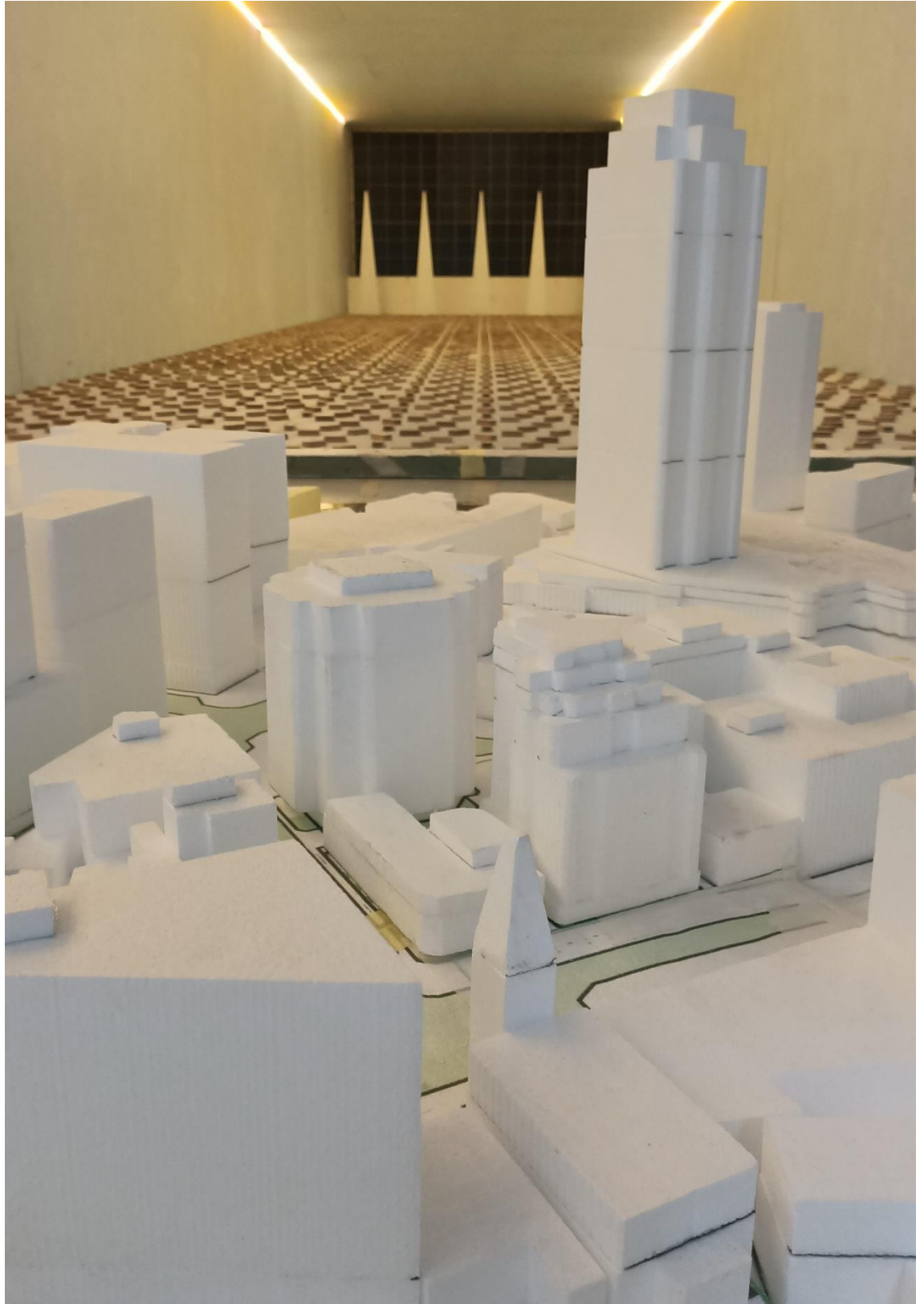
Figure 11: Photograph of the Wind Tunnel Model (Existing Site, view from the south-east)
