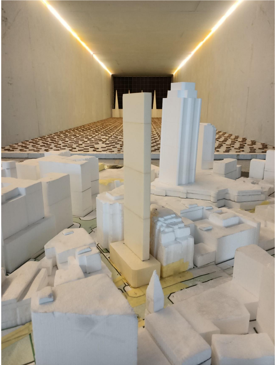
Figure 1g: Photograph of the Wind Tunnel Model (Base Case Massing, view from the south-east)
