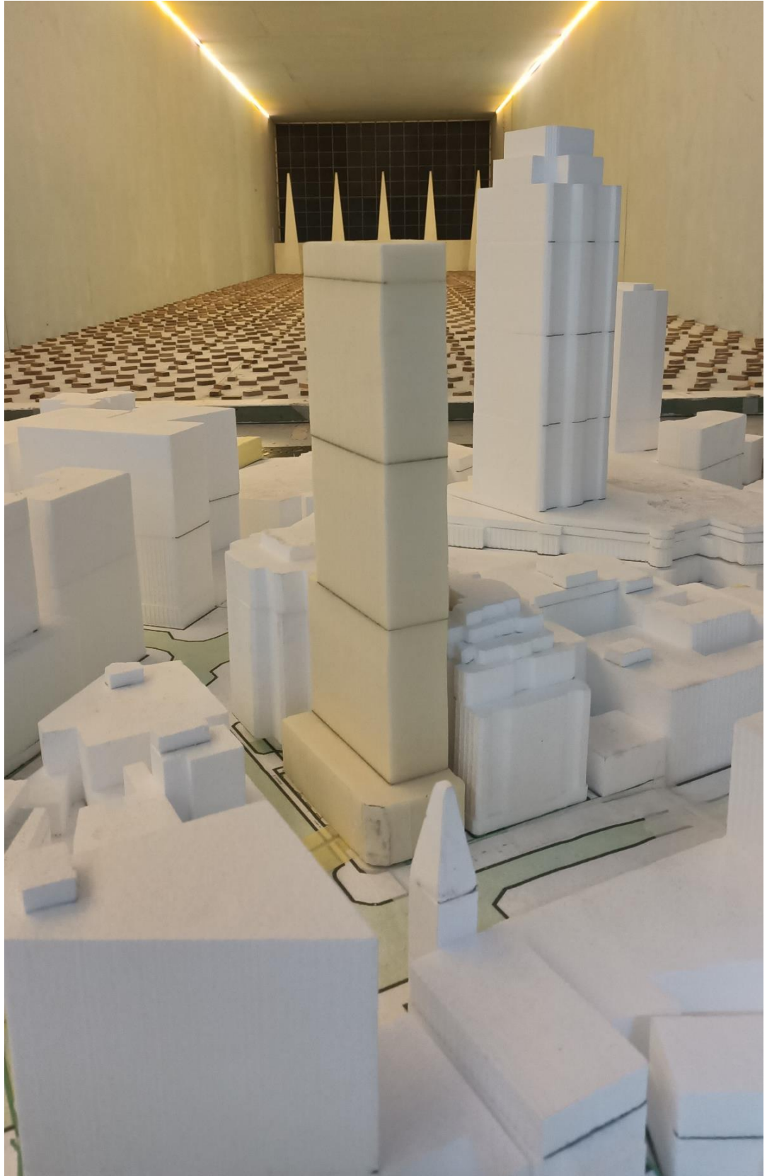
Figure 1j: Photograph of the Wind Tunnel Model (Alternative Envelope B, view from the south-east)
