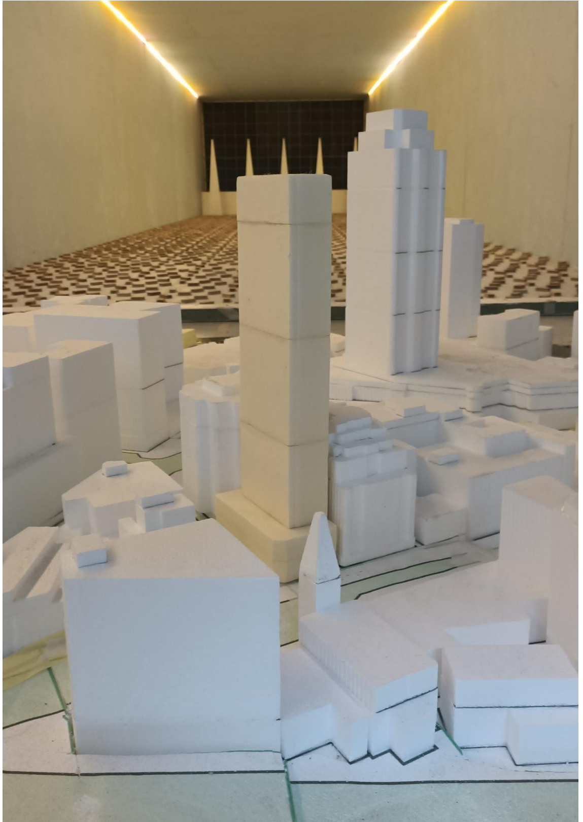
Figure 1h: Photograph of the Wind Tunnel Model (Proposed DCP Envelope, view from the south-east)
